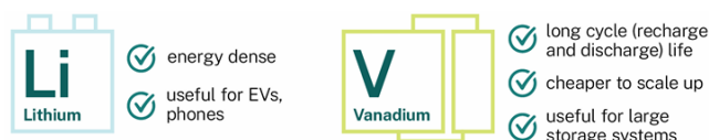
Figure 3 Australia's National Battery Strategy (2024), distinguishing advantages of lithium-ion batteries and vanadium flow batteries.
